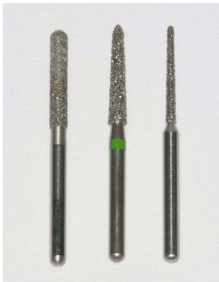
► Fig. 16.186 Cutting diamond instrument set for preparation. Different cutting diamond designs are available for shaping the crown stump. Based on the frequently used chamfer, a torpedobur (medium form) is most convenient.
